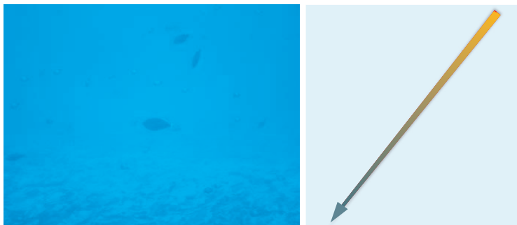
Figure 4: Light propagating through clear, absorbent media (left) continues in a straight line, but loses intensity (and may change color) with distance (right).
